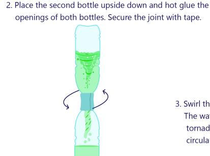
3. Swirl the filled bottle in circular motion and flip it. The water will drain in the empty bottle. See the tornado come alive with the swirl crated with circular motion.
